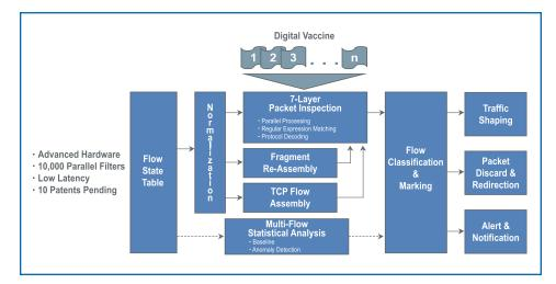
The TSE architecture also enables traffic classification and rate shaping. Sophisticated algorithms baseline "normal" traffic, allowing for automatic thresholds and throttling so that mission critical applications are given a higher priority on the network.
