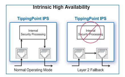
management engines. If an internal error is detected, TippingPoint can automatically or manually fall back to a simple Layer 2 device, configurable per segment. Additionally, TippingPoint offers a Zero Power High Availability (ZPHA) option for copper interfaces. In the event of full data center power loss, the interfaces can switch over to the ZPHA external relay to pass all traffic.
